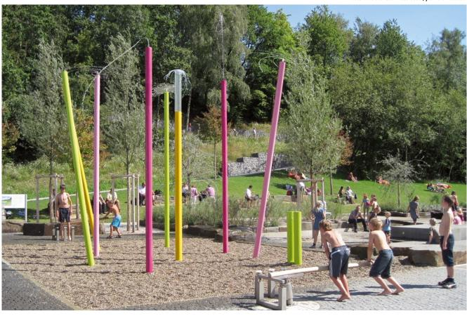
heads, the prevailing wind direction should be taken into consideration. The surfacing of the ground should be firm or graveled and be provided with a well working drainage. The water supply and the system must be drained during frost periods. Sensitive parts such as pump valves must be removed and stored in a frost-free location.
